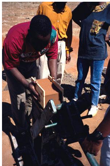
Figure 1: Brick moulding, Zimbabwe. Photo: Practical Action / Theo Schilderman.
