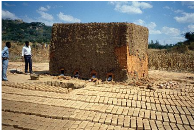
Figure 3: Coal fired bricks drying in sun Zimbabwe. Photo: Practical Action / Theo Schilderman.
